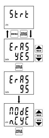
If it is needed to clear the memory before logging start, first it is necessary to select menu item logging START (symbol Strt) and confirm by pressing ENTER key.
